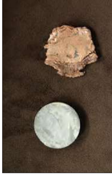
Comparison of a disseminated copper ore (left) and a piece of native copper (right). Disseminated ore bodies have a small amount of metallic mineral by volume.
